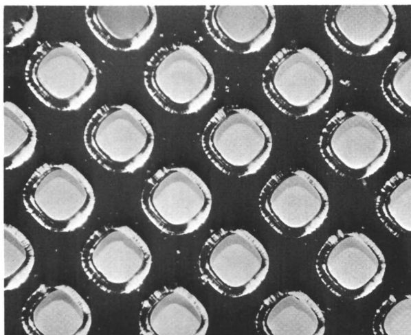
Figure 2. Mesh coated with poly(chloro-p-xylylene). Polymer is transparent inner rings. 16.5 ×
